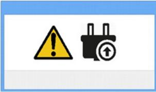
The Power Pack run time is now very limited. In order to protect the battery against deep discharge, the COW Controller will force the PC to shut down after a few minutes. The COW Controller will go into sleep mode and the status LED at the front of the Power Pack will go out. The battery will not undergo any further discharge. All it requires is to connect the Power Pack to the mains supply again to reactivate the COW Controller.
